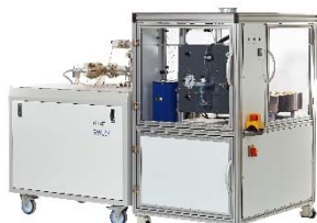
Figure 2. SPINMAS coupling with Robotic System and quadrupole mass spectrometer
