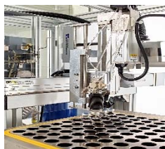
Figure 1. SPINMAS automatic coupling with sample changes
